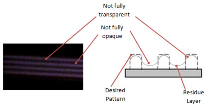
Figure 6: The IDT pattern on the mask and the profile effect from grayscale.
