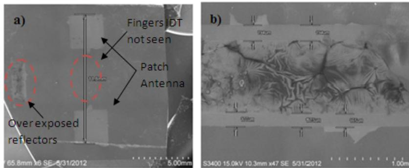
Figure 5: The SEM analysis of the pattern after lift-off process: (a) full view of the device and (b) the overexposed reflectors.
