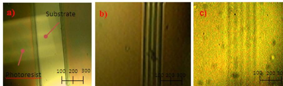
Figure 4: Optical microscopy images of development for: (a) 45 s, (b) 40 s and (c) 35 s.
