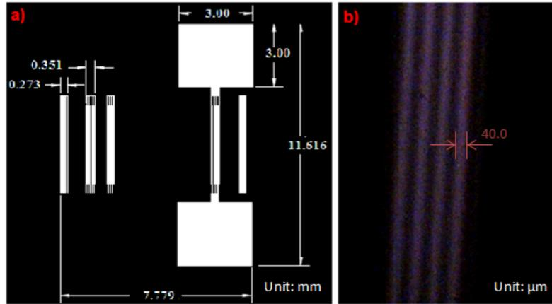
Figure 2: Illustrations of: (a) schematic of device and (b) the IDT finger from original mask.
