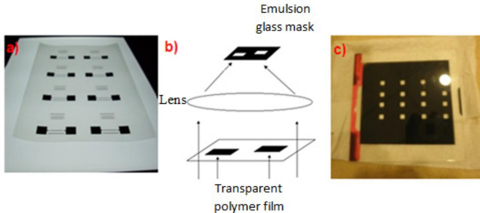
Figure 1: The mask-making process: (a) the patterned transparent polymer film, (b) the schematic of mask exposure system, and (c) the result; negative of emulsion glass mask.
