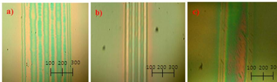
Figure 3: Optical microscopy images of the patterned IDT structure using UV dosages of: (a) 369.2  $\text{mJ cm}^{-2}$ , (b) 390.5  $\text{mJ cm}^{-2}$  and (c) 404.7  $\text{mJ cm}^{-2}$ .
